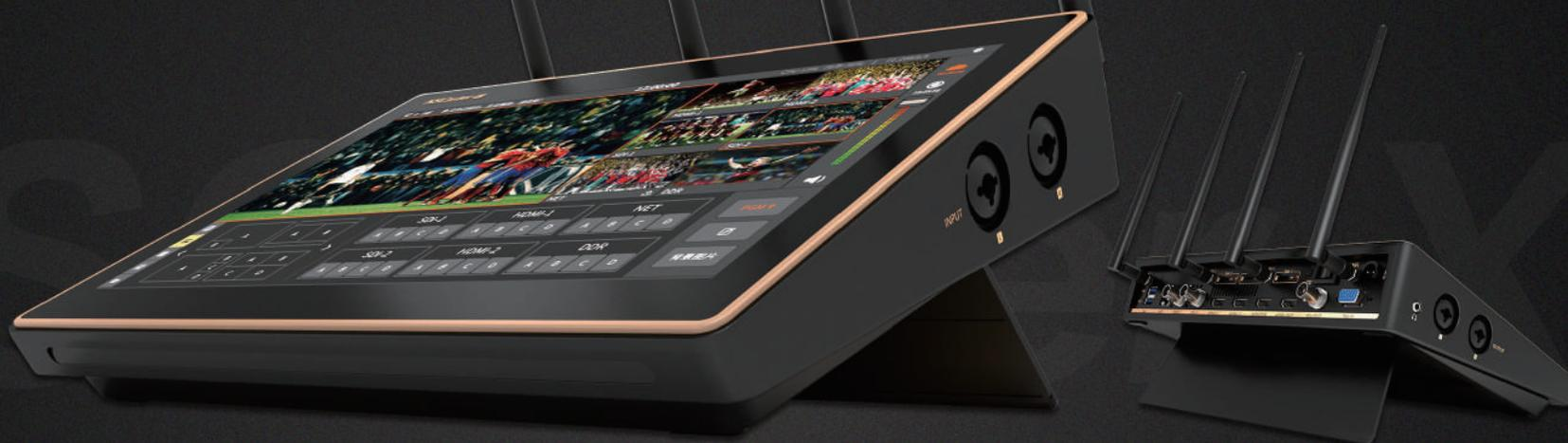
NSCaster X1 4G bonding version is a highly integrated navigation tablet with a built-in 11.6-inch full HD touchscreen monitor. It integrates functions such as multi-channel switching, recording, broadcasting, audio mixer, special effects, and monitoring. It also has built-in Ethernet, WIFI, and 4G bonding modules to meet the needs of webcasts for different scenarios .
