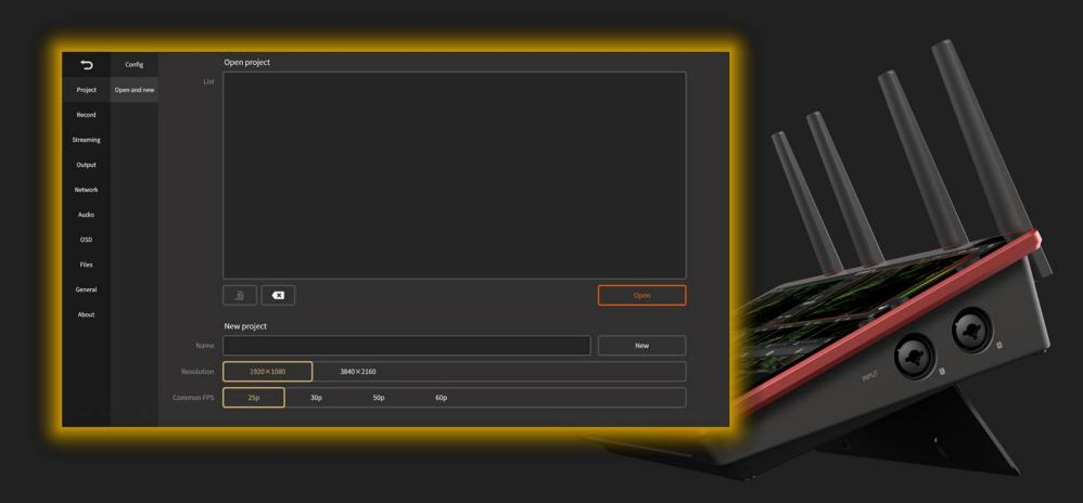
**NSCaster X2** can setup the project, establish the project name, resolution and bit rate. Complete the program production in projects.
