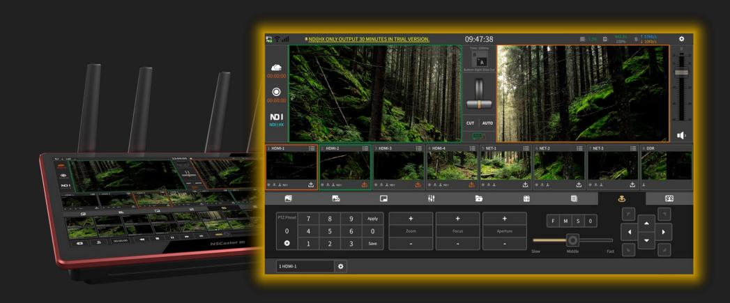
**NSCaster X2** has a built-in PTZ control interface and supports a variety of mainstream PTZ control protocols (visca over IP, onvif, NDI|HX). It can remotely control the camera PTZ, supports zoom, focus and aperture control, supports up, down, left, right, top left, bottom left, top right and bottom right PTZ movement, supports PTZ movement by knob, and quickly locating the target position.
